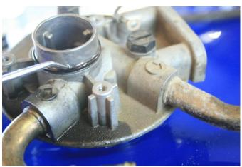
Step 3: Turn housing over and remove the two #20 torx bolts.
