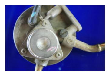
Step 2: Replace with the largest o-ring provided. Re-install pump cover with the 3 #20 torx bolts.
