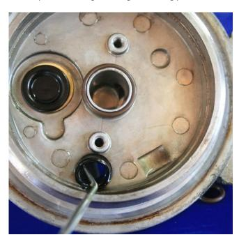
Step 7: Replace smallest o-ring on bleeder screw with o-ring provided.
